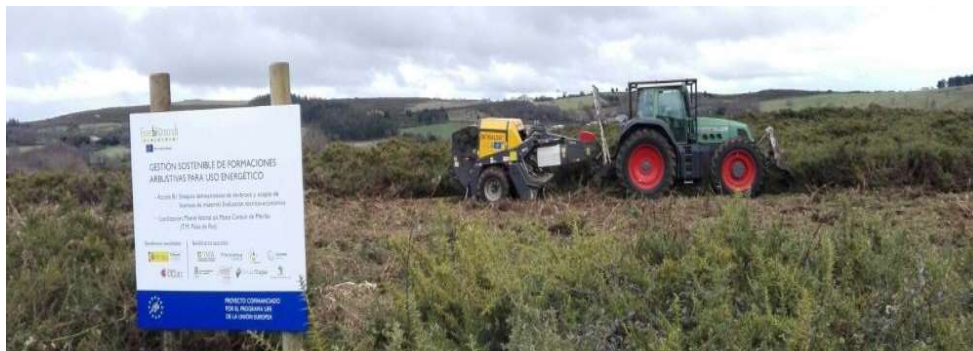
Demonstrative mechanized collection of brush biomass in Spain (Enerbioscrub Life + Project)
