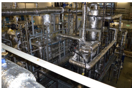
Pilot facility for the production of 1 barrel per day of Fischer-Tropsch raw product at BEST – Bioenergy and Sustainable Technologies (former BIOENERGY 2020+ GmbH), Austria.
