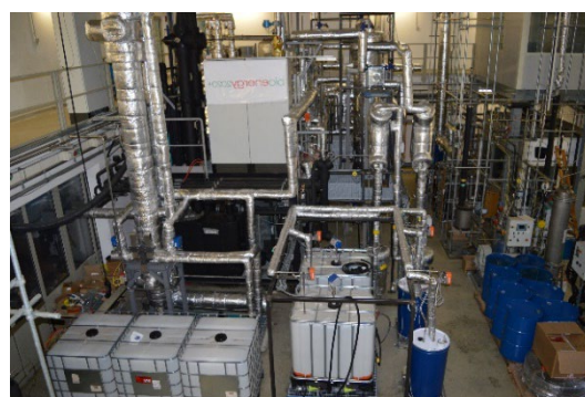
Pilot facility for the production of 1 barrel per day of Fischer-Tropsch raw product at BEST – Bioenergy and Sustainable Technologies (former BIOENERGY 2020+ GmbH), Austria.
