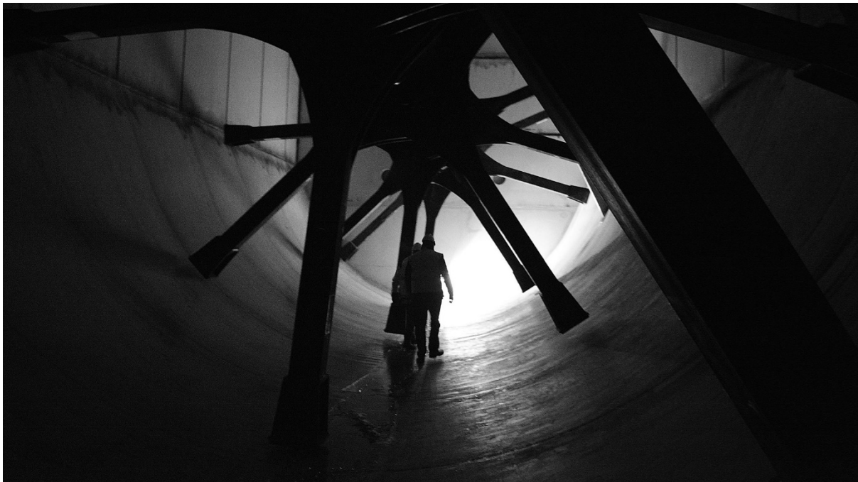
Picture from the inside of a plug flow reactor. During operation, the agitator is rotating along a center shaft. Credit: Daniel Tamm
