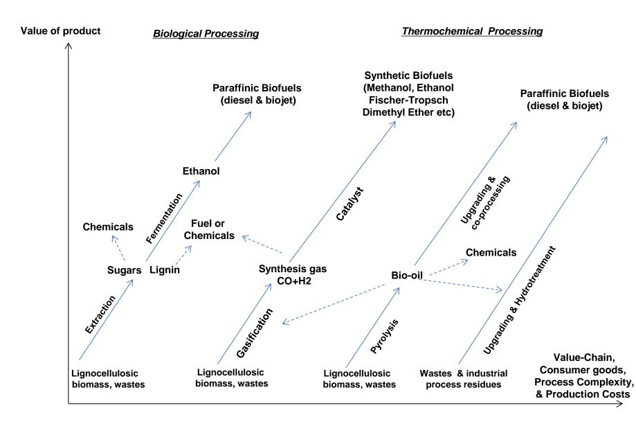
Adding value to biomass by processing to advanced biofuels and to biochemicals
