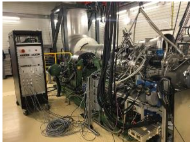
100%SAF helicopter engine ground test (2021)
