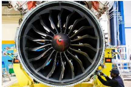
100%SAF ground test of LEAP engine and in-flight demo A320 Volcan project (2021 - 2022)
