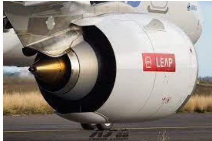
100%SAF ground test of LEAP engine and in-flight demo A320 Volcan project (2021 - 2022)
