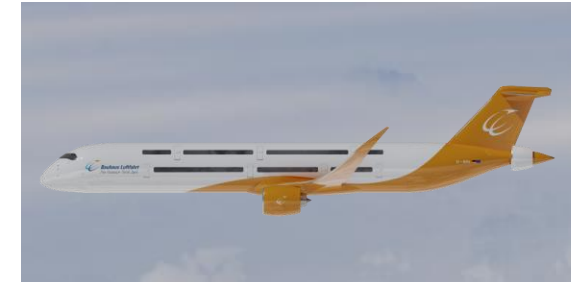
Long-haul LH 2 aircraft Liquid hydrogen powered long-haul aircraft, twin-gas turbines
