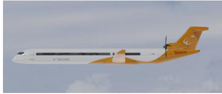
Regional LH 2 aircraft Liquid hydrogen powered regional aircraft, Fuel-cells / propellers
