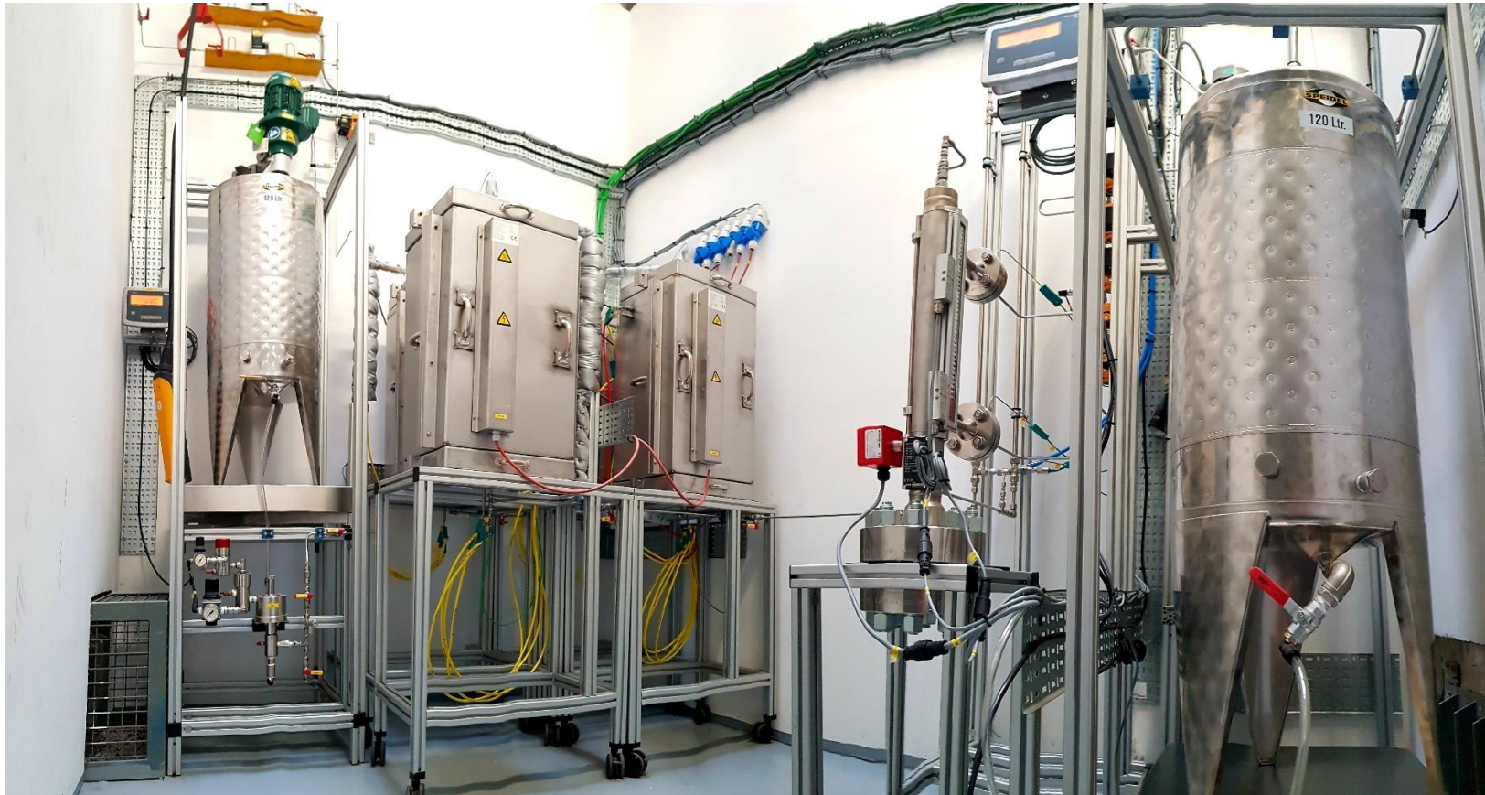
50 kg/day catalytic hydrotreater
