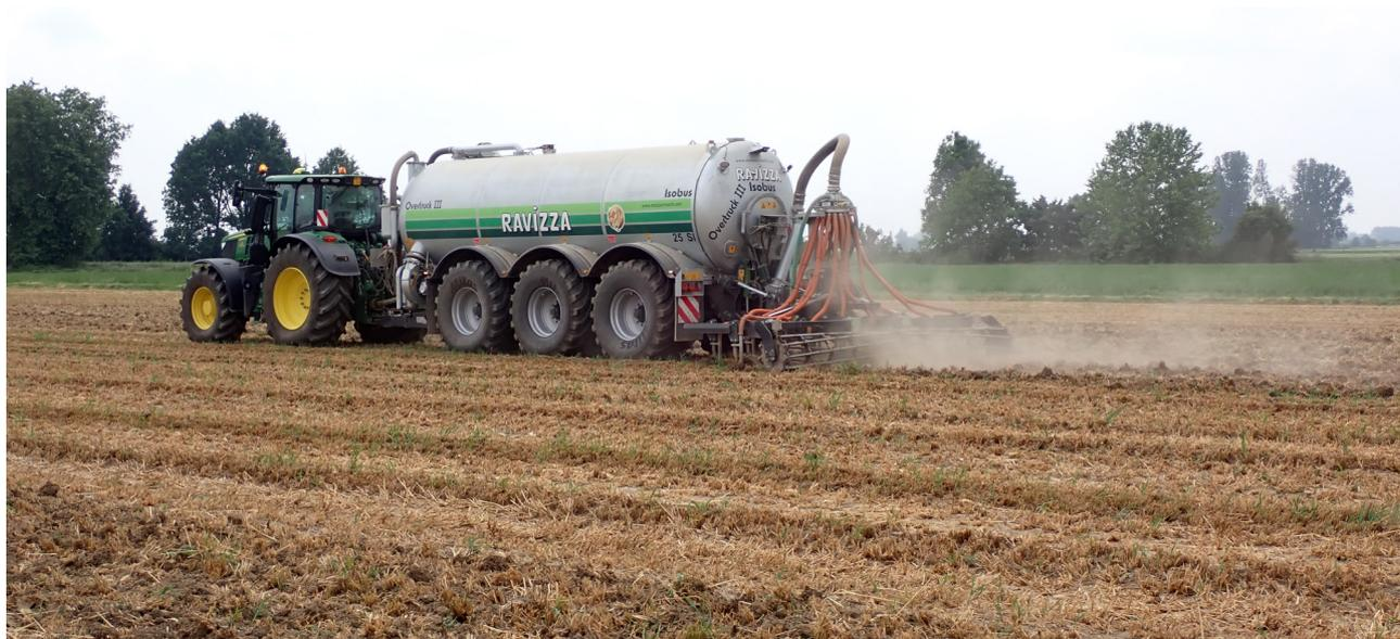
Figure 3. Biogasdoneright strip till digestate application (Italy). © Peter Kornatz
