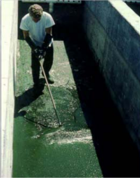
Figure 39: Harvesting of microalgae by sedimentation (Lundquist (139) )
