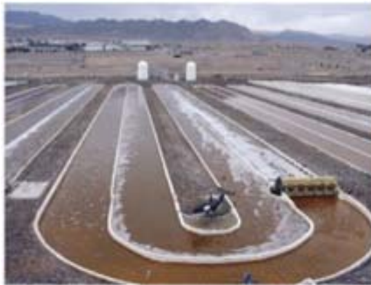
Figure 3: Raceway pond used for the production of Dunaliella salina in Israel (Wijfels (245) )
