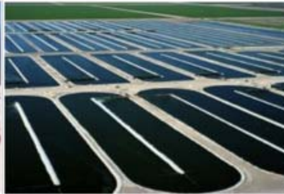
Figure 2: Raceway ponds used for the production of Spirulina platensis in California (Borowitzka (29) )
