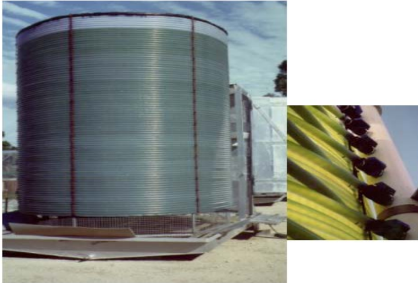
Figure 11: A one thousand liter, pilot scale helical photobioreactor in Australia (BEAM (11) ).
