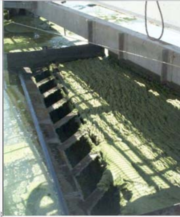
Figure 40: Harvesting of microalgae by flocculation – floatation (Lundquist (139) )
