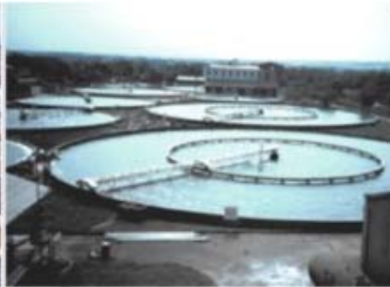
Figure 4: Circular ponds used for the production of Chlorella sp. in Japan (Borowitzka (29) )
