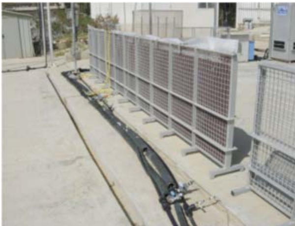
Figure 12: Vertically oriented flat panel photobioreactor at Ben Gurion University of the Negev, Israel (Wijffels (245) )
