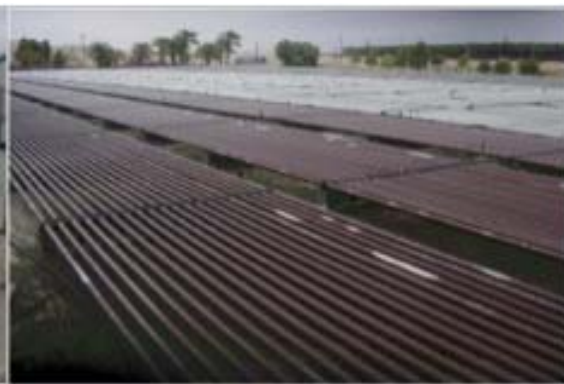
Figure 7: Horizontal, tubular photobioreactor at Algatechnology, Israel (Wijfels (245) )
