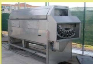
Limonene removal equipment
